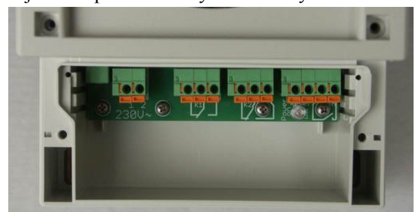
Electrical terminals of prh-ZG4
